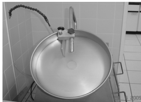
Figure 2: Rotation dish granulator used for grain preparation of clay and urea.
